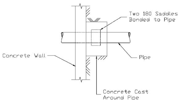
**Figure 3** - Detail of Anchor Restraint at Wall and Manhole Penetrations in Buried Systems
