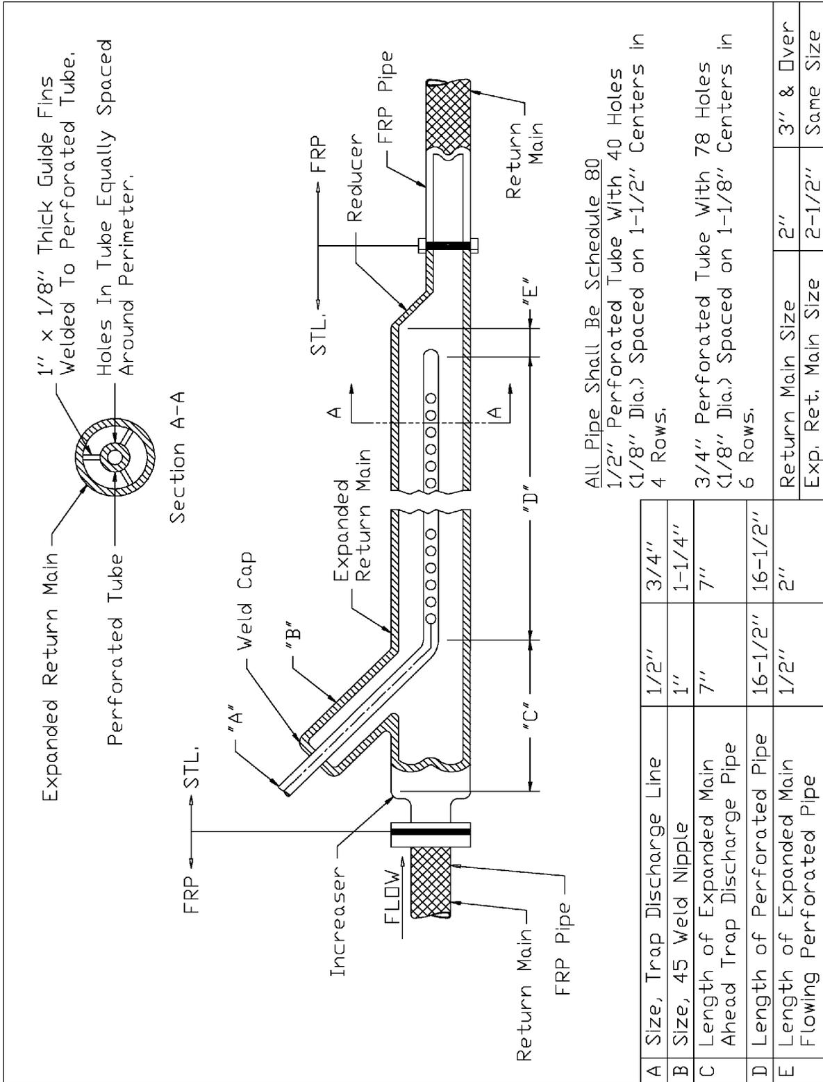
**Figure 2 - Detail for Typical In-line Steam Dissipation Chamber at a Trap Discharge Connection**
