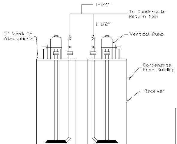
**Figure 1** - Typical Hot Well for Pumped Condensate Return
