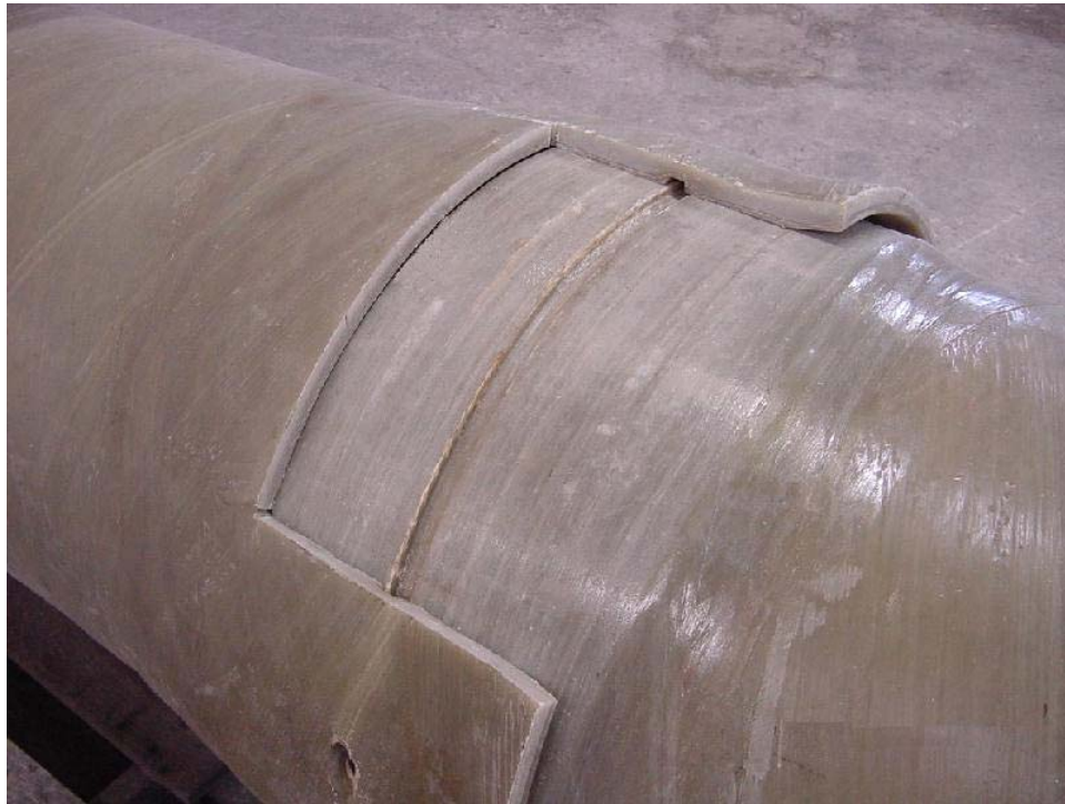
24" diameter Kwik-Lock joint, after high pressure testing - This joint was cut away to examine the grooves and laminate for stress assessment
