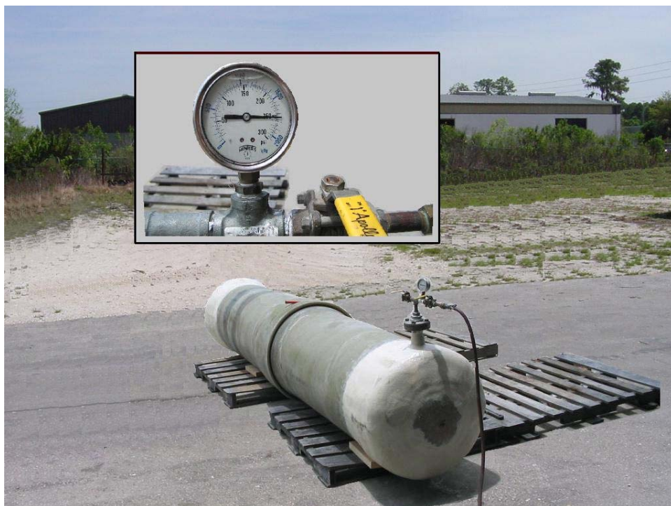
Testing of our 24" diameter single O-ring joint was done to 250 psi with no leaks.
