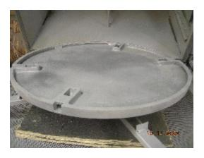
**The Challenges:** The hybrid steam manhole covers require a strong bond between the high strength composite laminate and the cast iron dish. Extensive bond tests were performed to check the strength of the laminate and adhesion to the cast iron cover. The final product uses a locking key to enhance the bond of the FRP composite to the cast iron. The end result is a FRP hybrid manhole cover that withstands heavy traffic loads.
