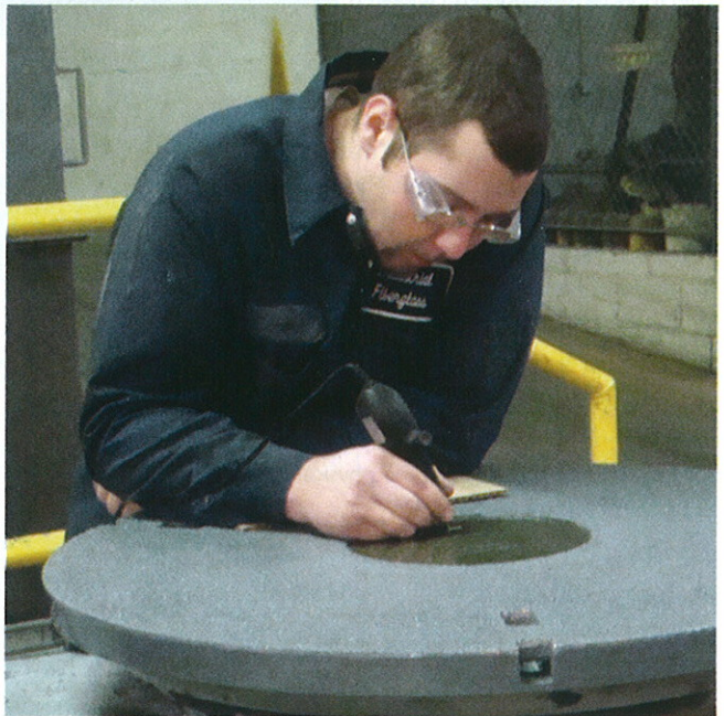
A serial number is engraved into each part before shipping.
