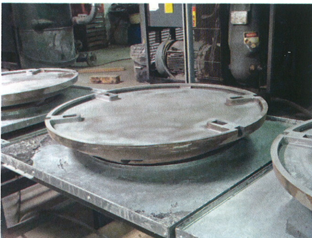
Production starts by grit-blasting a cast iron 'dish'.
