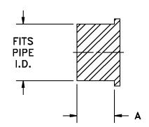
Plug fits pipe I.D. State pipe I.D. or manufacturer. Refer to Fig. #11 for sizes larger than 4".
