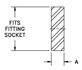
Plug fits fitting socket. Larger sizes available on request. Fitting plugs to size 6" are rated for 150 psi working pressure. Sizes 8" through 12" are reduced to a rated working pressure of 75 psi.
