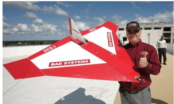
On display by CESI for all the local, State and Federal dignitaries at the grand opening was the next generation UAV, which had been partnered with FiberSystems. This latest version of the UAV utilizes all carbon fiber reinforced composite radar invisible stealth technology and construction for the UAV body.
