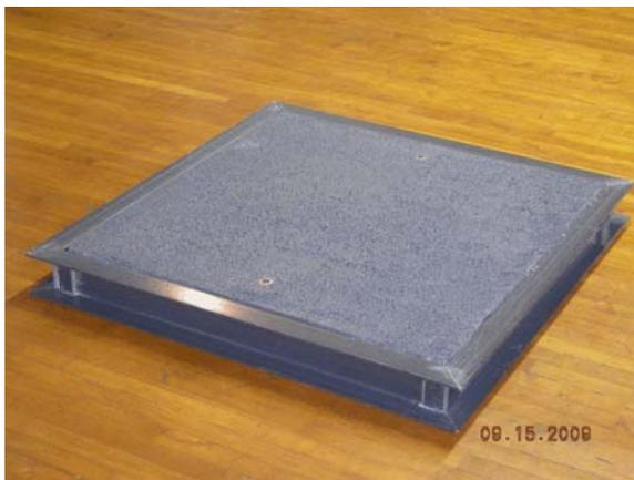
The requirement was added that the 36" x 36" manway cover would also have to take H- 20 live load (32,000 lbs.). At the same time the FRP cover would be required to handle the 200° design temperature on the bottom of the cover. The temperature on the top of FRP cover would need to be less than 140° - so that no one would be burned if they stepped or fell on the cover.
