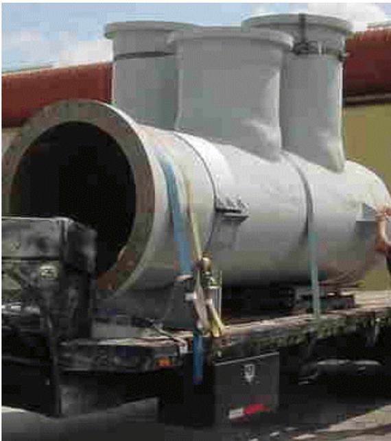
**The Solution:** FiberSystems provided the customer a "turn key" package - including finite element analysis (FEA) engineering, the long "trouble free" service life of CorBan FRP composite factory assembled isometric spools, and the new pipe supports. For the FEA engineering, Algor's Pipe Pak was used by FiberSystems.
