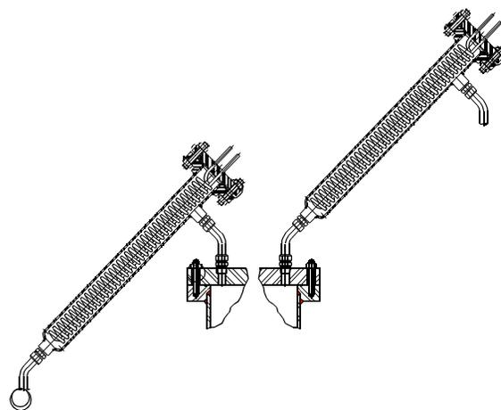
Condensers may be used to remove or recover overhead vapors. Condensation may recover vaporized reactants, products or solvents, or the return of liquid as reflux. Coil in shell condensers with removable coils can be mounted for recovery or reflux operation.
