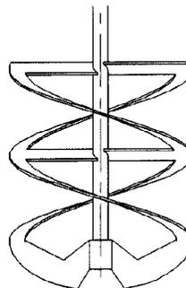
Special manufacturing techniques assure uniform pitch and close clearances for high performance and accurate scalability to larger reactors.
