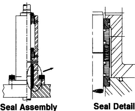
Single, dry-running mechanical seals are a less expensive option for some lower pressure applications.
